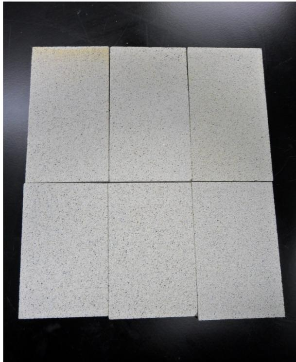
Accelerated aging coupons of polyester polymer concrete test (control samples on bottom) – Kreysler & Associates Kastone finish at 2500 hours QUV exposure
